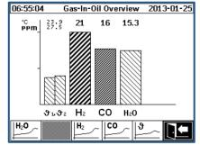
Individual chart diagram for Hydrogen (H<sub>2</sub>), Carbon Monoxide (CO), Moisture in Oil (H<sub>2</sub>O) and temperatures.
