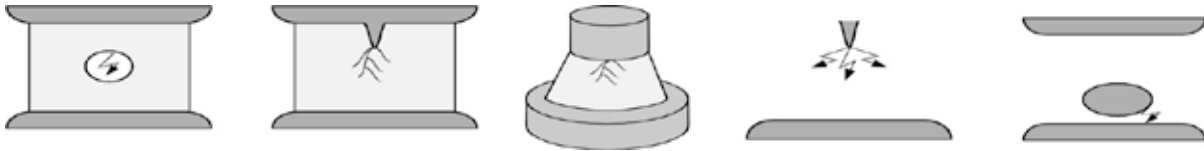
Example Sources of Partial Discharge
